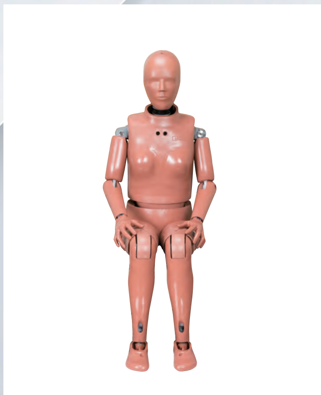
Light weight Hybrid-III 5th Percentile Female Dummy (20 kg)
